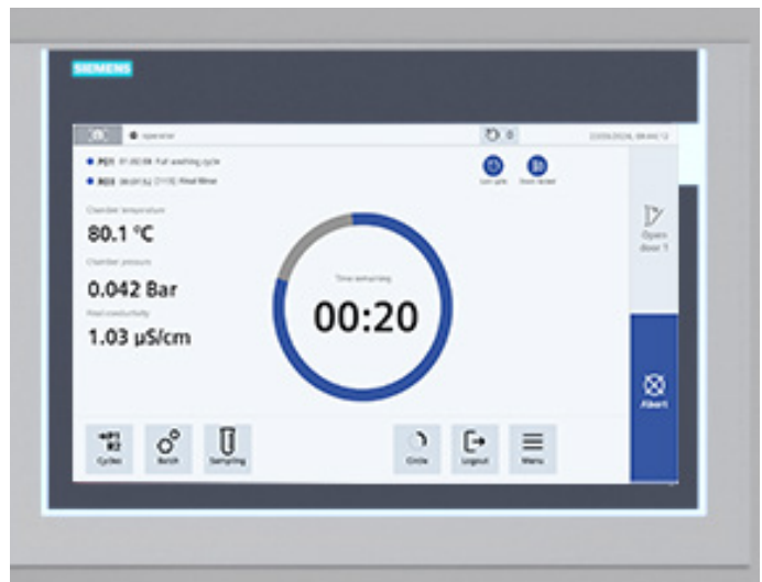
The Siemens - Simatic (S7 Based platform) control system incorporates an intuitive touchscreen interface that provides reports, control options and real-time system monitoring.
